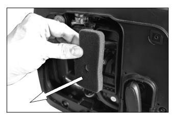
engine oil and squeeze the filter to remove excess oil.
