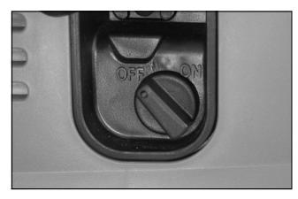
3. Turn the air vent knob to the 'Close' position.
